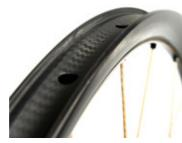
**TECHNICAL DETAILS RIM** Rim Material Carbon Spoke holes 24 Inner width 25 mm Height 27,5 mm Tire range 28 mm - 61 mm Finish UD **Profile** Asymmetric rim profile Tubeless ready Yes **Hookless** No
