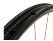
**TECHNICAL DETAILS RIM** Rim Material Carbon Spoke holes 28 Inner width 30 mm **Height** n. a. Tire range 2,2" - 2.7" Finish UD **Profile** Symmetric rim profile Tubeless ready Yes **Hookless** Yes Rim weight 265g
