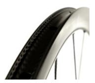
**TECHNICAL DETAILS RIM** Rim Material Carbon Spoke holes 24 Inner width 25 mm Height 36 mm Tire range 28 mm - 61 mm Finish UD Profile Asymmetric rim profile Tubeless ready Yes
