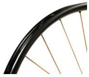
**TECHNICAL DETAILS RIM** Rim Material Carbon Spoke holes 24 Inner width 25 mm Height 27.5 mm Tire range 28 mm - 61 mm Finish UD Profile Asymmetric rim profile Tubeless ready Yes Hookless No
