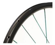
**TECHNICAL DETAILS RIM Rim Material** Aluminium Spoke holes 24 Inner width 25 mm Height 25 mm Tire range 28 mm - 61 mm Finish Brushed **Profile** Asymmetric rim profile Tubeless ready Yes Hookless No
