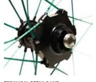
**TECHNICAL DETAILS HUB** Disc mount standard Centerlock Spoke holes 24 **Axe width** 12 x 100 / 12 x 142 Hub weight 388g front / 196g rear
